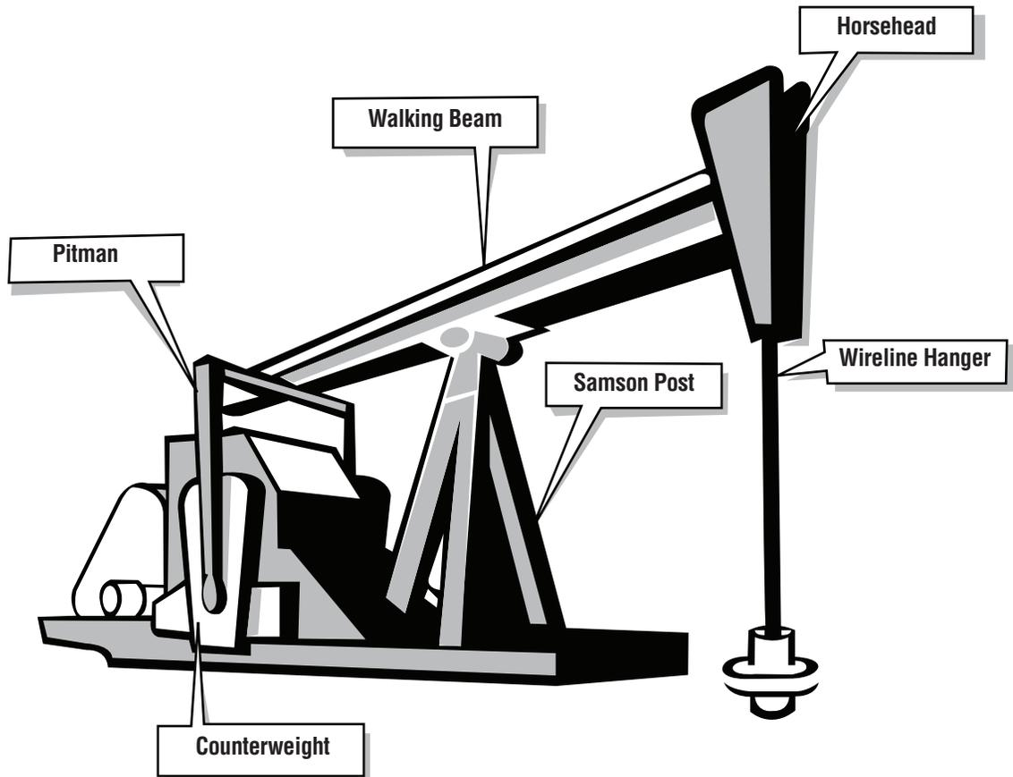
Artificial lifting systems, or pumping units, are used to help pull the oil out of the reservoir rock and pump it up the well. A down hole pump in the well is connected to the pumping unit by steel rods, which are screwed together. The pump is activated from the up and down movement of the pumping unit of the surface. As the pump plunges down, fluid from the rock formation flows into the pump chamber. On the upstroke, the fluid in the chamber is forced up the tubing, to the surface.
